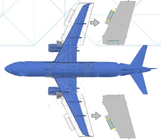
Wing dock configured for tail-in or nose-in
