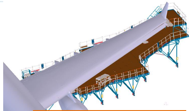
Modular Wing Dock on LH main wing
