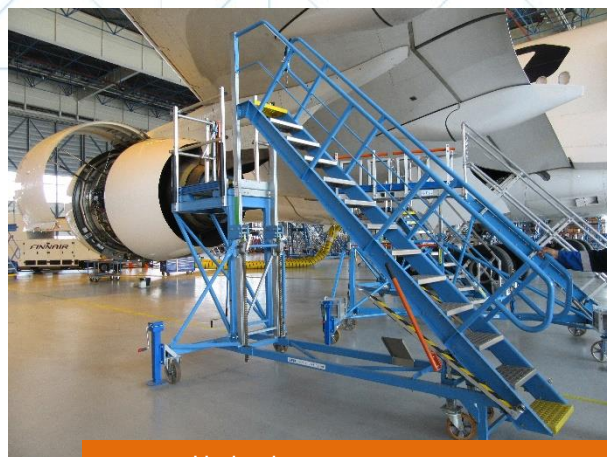
Under thrust reverser access
