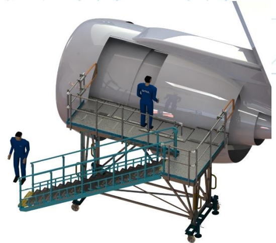
Under fan cowling access
