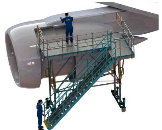
Access up to the engine pylon
