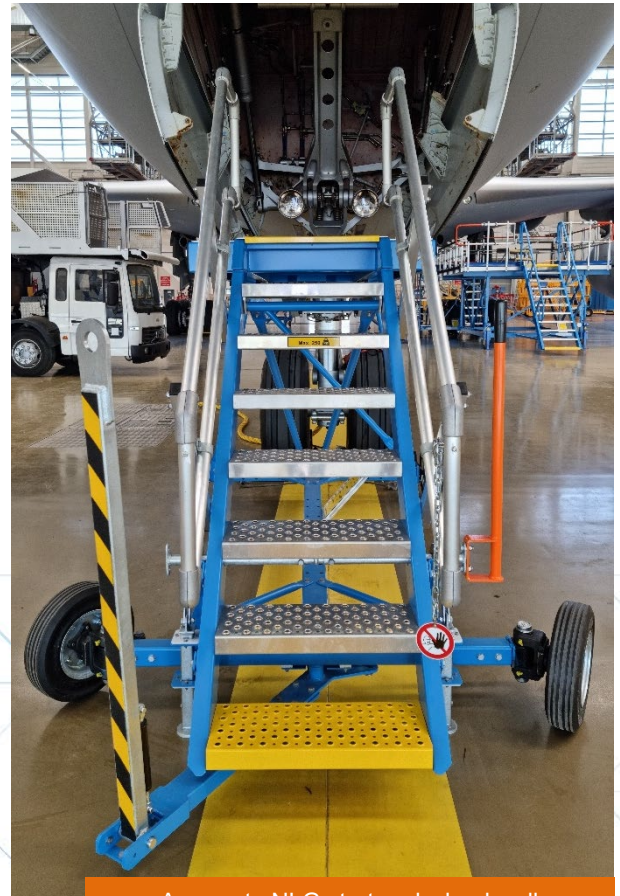
Access to NLG strut and wheel well
