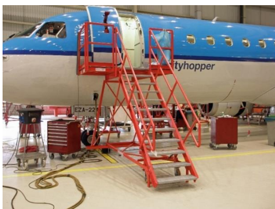
Fixed Height Stairs with large platform to access PAX Door
